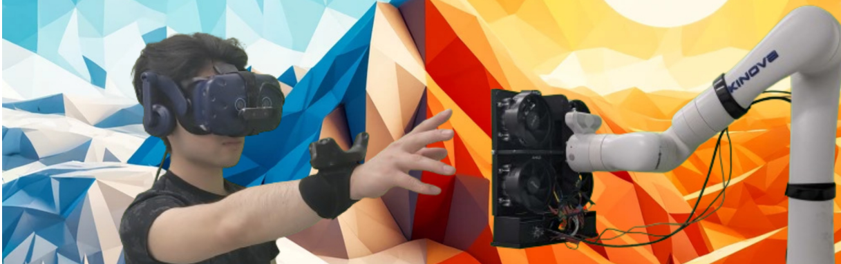
Figure 1: We introduce an Encountered-type Haptic Display that incorporates thermal feedback to enrich VR experiences, our study shows significant improvements in user immersion and haptic realism.
