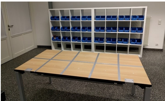
Figure 4: The setup that was used to conduct the user study. In the background there is the picking area containing of 48 picking pins. In the front is the placement area consisting of 10 placement spots
