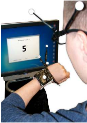
Figure 2: The setup of the controlled experiment with two retro-reflective apparatuses mounted on the participant's head and wrist and the display showing the current task.
