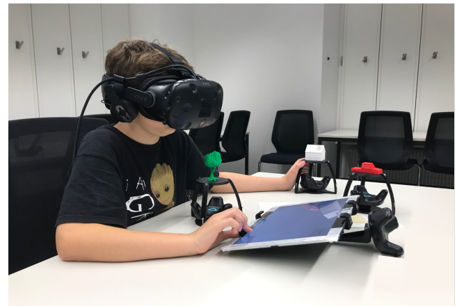
Figure 2: Study setup: a child is wearing VR glasses as an instantaneous output for the input provided by tangibles and a tablet. New virtual objects are created by placing tangibles on the tablet surface and can be modified via touch input.
