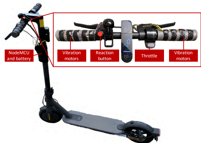
Figure 3: The E-Scooter was equipped with four vibration motors on the left and right sides of the handlebar and the reaction button on the left to measure reaction time to the warnings. The vibration motors and the reaction button were directly connected to a NodeMCU microcontroller for communication with a HoloLens.
