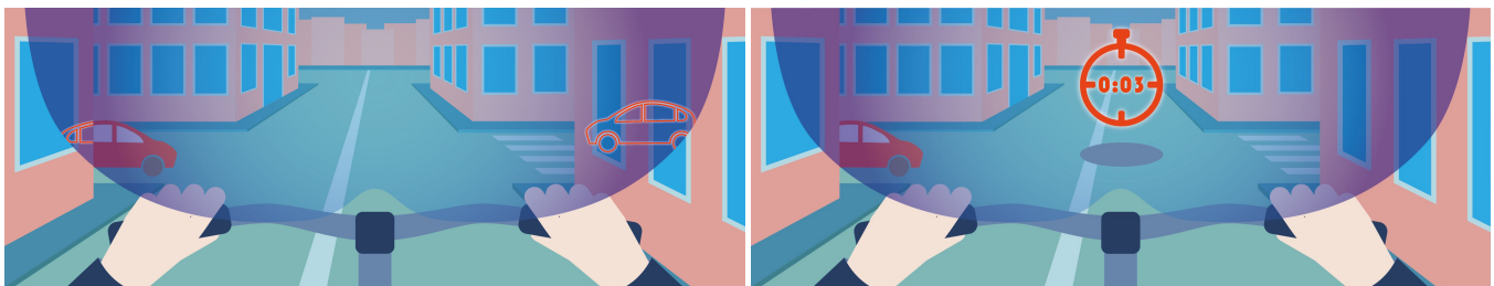
Figure 1: Overview of two visualization concepts to support cyclists' crossing decision-making at visually occluded urban environments: X-ray highlights occluded cars (left) and Countdown displays time the intersection remains safe to cross (right).
