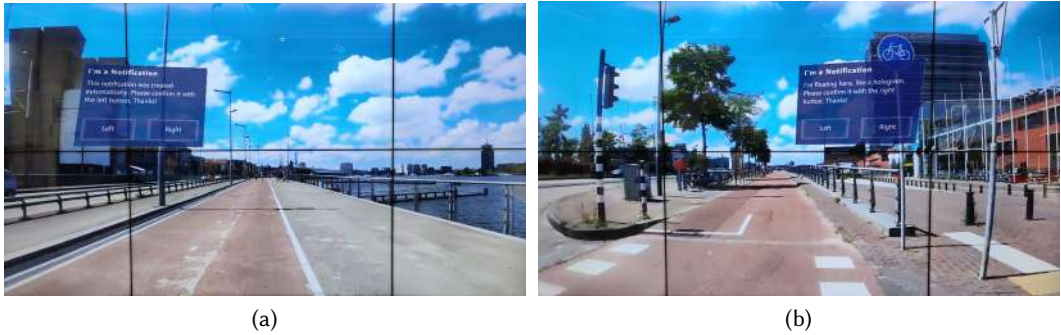
Fig. 3. Video wall simulating a cycling scenario while participants were receiving AR notifications using a HoloLens 2. All notifications contained a text, advising participants which button to press. (a) : Participants were inquired to select the left button. (b) : Participants were asked to press the right button.
