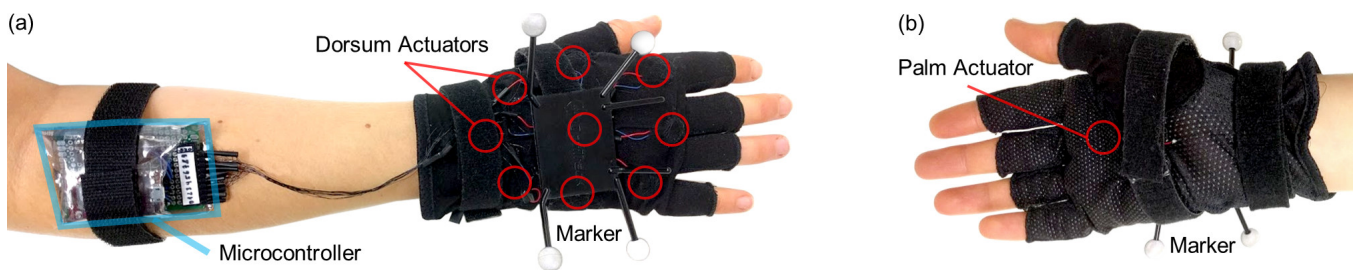
Figure 1: TactileGlove prototype showing the (a) dorsum, and (b) palm of a user's hand. Red circles highlight the positions of the vibration actuators and blue indicates the position of the microcontroller.
