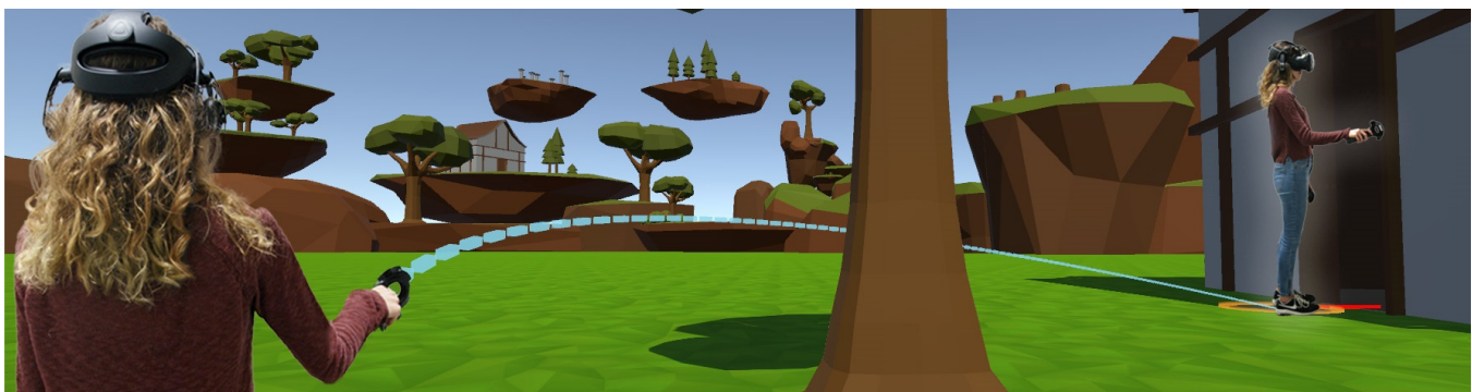
Figure 1: A user is teleporting herself in a Virtual Environment using the Curved Teleport . It allows her to teleport around an obstacle and graphically choose the orientation, which she wants to face after teleportation only by using the curved trajectory visualization with orientation indication, and without having to turn her body in the physical world.
