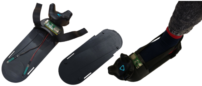
Figure 4. The inside of our prototype with two visible sensors (left), the top sole with the four pins (middle) and an example of how the prototype is worn (right)
