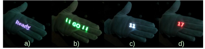
Figure 3: Visual feedback in the study: After reaching the starting position (a), the system showed the direction of interaction (b). The participants task was to browse through a stack of white colored numbers (c) to find the one red colored number (d).
