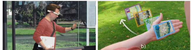
Figure 1: A map application as an example of one-handed (a) proximity-based interaction with a linear layered information space. The user can browse map layers by moving his hand through the space (b).
